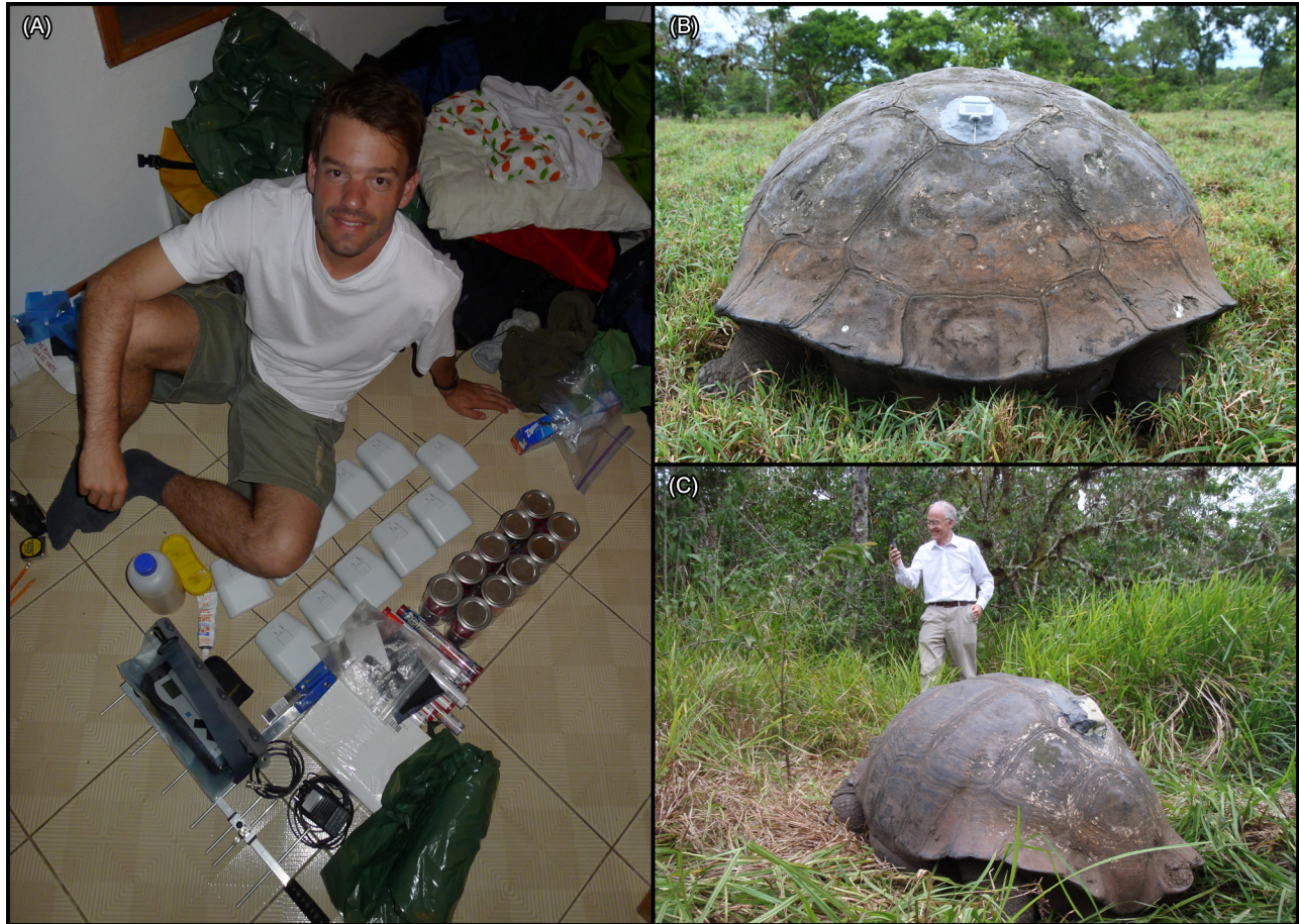
FIGURE 13.2 The first GPS tags deployed on Galapagos giant tortoises were made by Franz Kummeth and weighed approximately 500 g (A). Tags were fitted to either the front (females) or rear (males) of the carapace using plumber's epoxy putty (B). Tags stored many months of data, which could be retrieved with a handheld base station (C). Randall Keynes (Charles Darwin's great-great-grandson) downloading movement data from an adult male who could very well have been alive and migrating when Darwin was writing his masterwork. GPS , Global positioning system. Photos: Stephen Blake.
